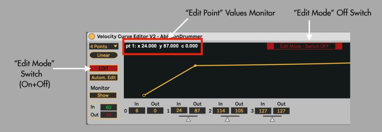
Switch on "Edit Mode" to edit the individual points by mouse drag. When hovering over a point the values of this point will be shown at the top. Make sure to switch off "Edit Mode" after you finished editing.
