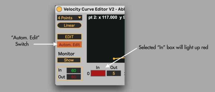
Switch on "Autom. Edit" and then select the "In" number box you want to edit, a selected number field will light up red. Then play/hit/ press the MIDI note (e.g. via your external controller). The velocity value of this note will be automatically detected and set to the number box.
