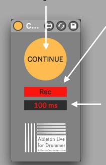
Switch on "Rec" to have "Arrangement Record" automatically activated when CONTINUE playback is triggered.
